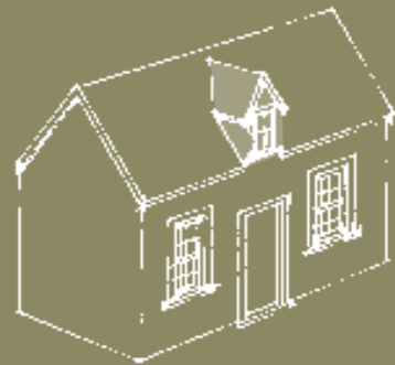
roof space developed and dormer window added
