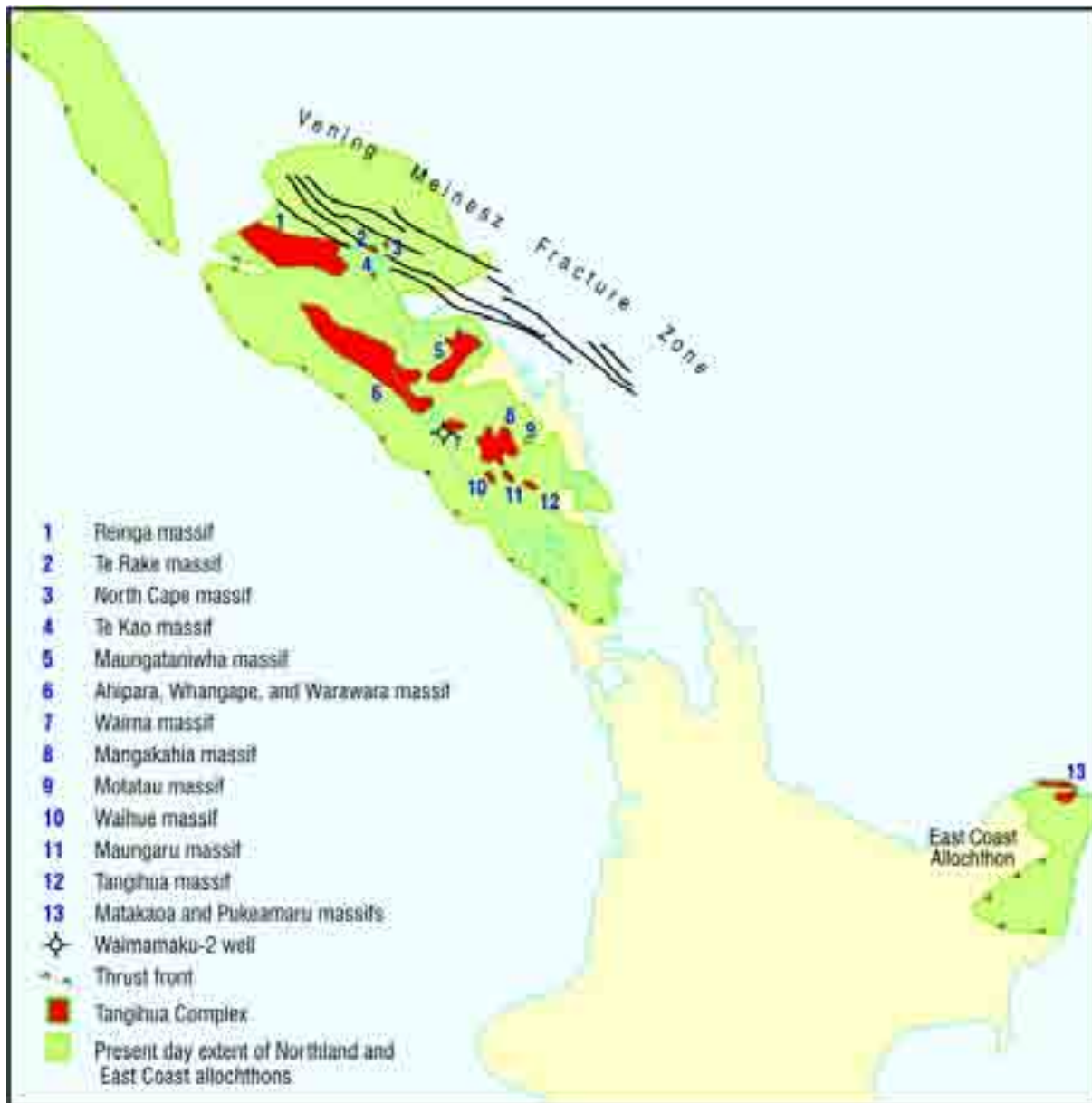
Figure 12. The Northland Allochthon extends west of Northland and as far south as Auckland. The East Coast Allochthon is a correlative. Much of the Northland Allochthon has been eroded. The major Tangihua Complex massifs are numbered and named (after Fig. 4.1 of Isaac et al. 1994).
