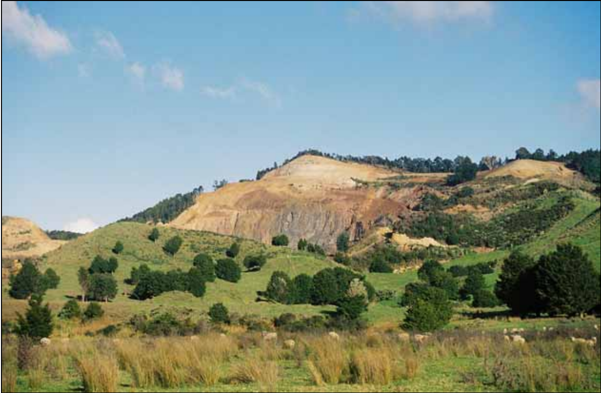
Figure 18. Puketona quarry northwest of Paihia. The quarry is operated by McBreen Jenkins Construction Ltd and produces both greywacke and basalt aggregate. Photo: Tony Christie.
