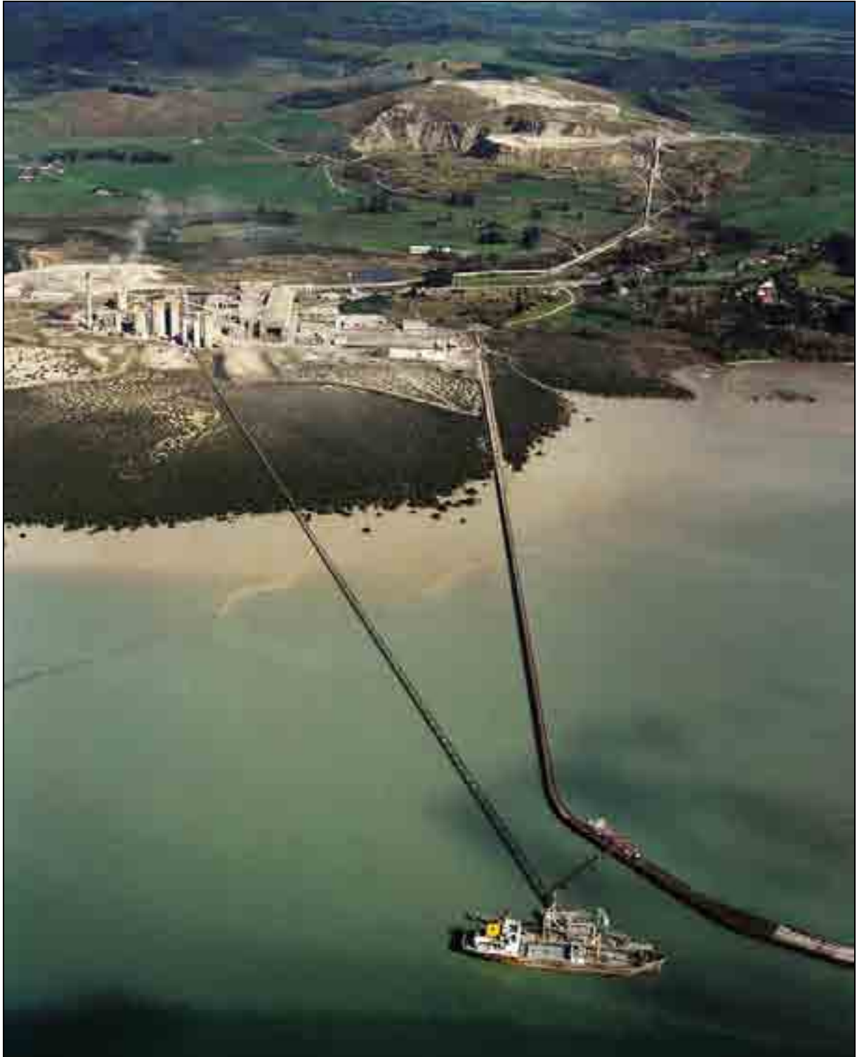
Figure 25. Golden Bay Cement's limestone quarry and plant at Portland, 8 km south of Whangarei. The plant has an annual production capacity of 600,000 t. Cement is shipped to eight distribution centres throughout New Zealand and approximately 20% is exported to Tahiti and other Pacific Island countries. Photo: Lloyd Homer CN26655/12.
