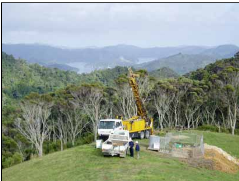
Figure 44. Drilling on Aurora Minerals Hazelbrook epithermal gold-silver project area. A. RAB (rotary air boring) drilling soil samples. B. Reverse circulation drilling with cyclone separator (white) near centre and bagged samples in the foreground. C. Diamond drilling - core drilling with a diamond bit. Photos: courtesy of Aurora Minerals.
