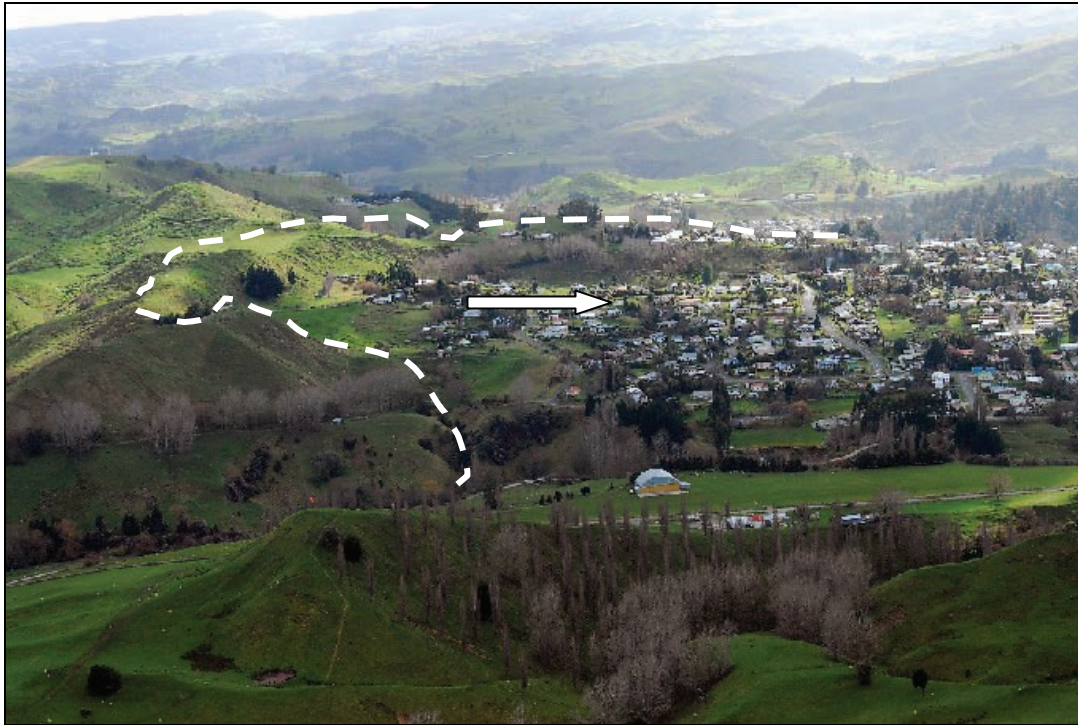
Figure 2.5 Translational landslide, Taihape. Arrow shows the direction of slide, with line showing the headscarp area. Photo: G.T. Hancox, GNS Science.
