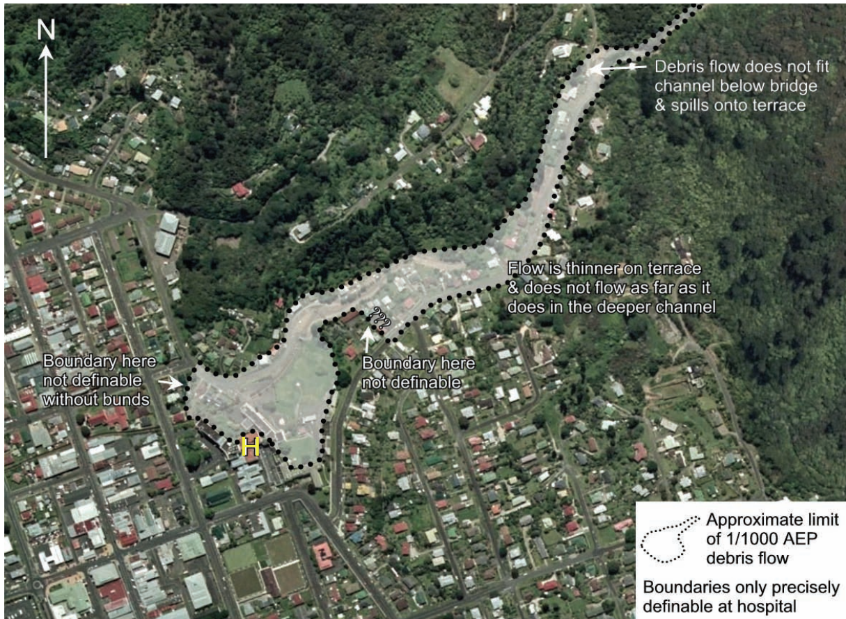
Figure 4.2 Example of a landslide hazard assessment including risk. The annotated aerial photograph depicts the 1/1,000 AEP debris flow hazard zone at Karaka Stream, Thames, Coromandel, in relation to existing BIC 3 buildings in the Thames Hospital complex (H).
