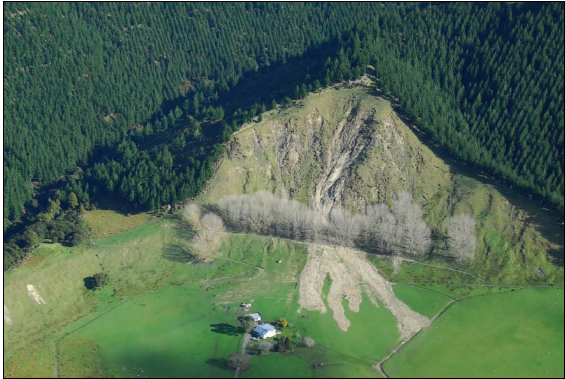
Figure 2.3 Earth slide in regolith and rapid debris flow in the run-out zone, north east of Wanganui at Mangamahu, during the July 2006 rainstorm. Photo: G.T. Hancox, GNS Science, July 2006.
