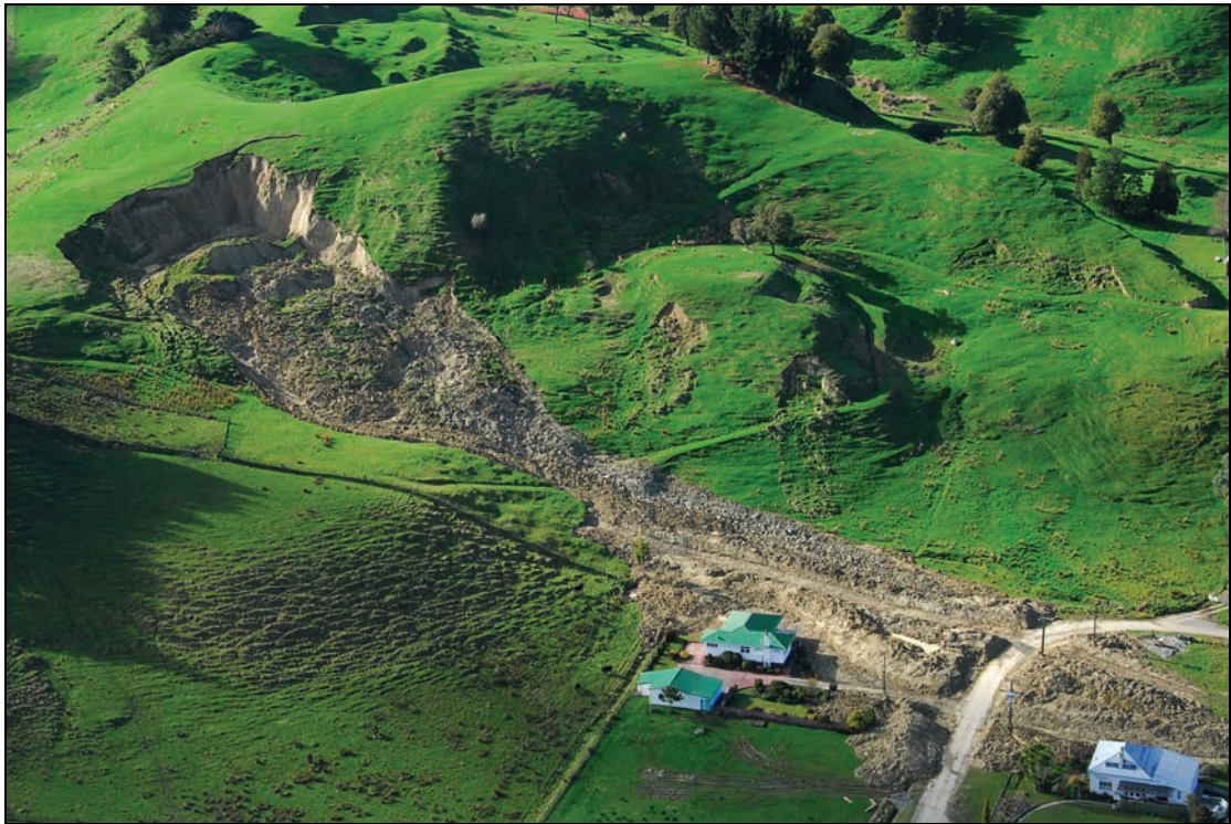
Figure 2.4 Deep-seated rotational slide in mudstone (left) and slow-moving earthflow in the toe area (right), which occurred at Hunterville during the July 2006 rainstorms, causing the temporary evacuation of four houses. Photo: G.T. Hancox, July 2007.
